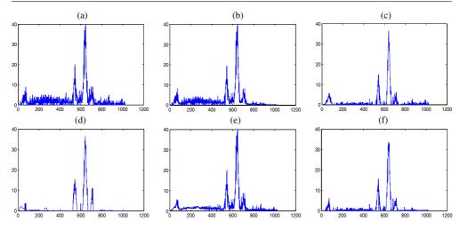
**Figure 6.** Typical single-pixel spectra of the Cr/Fe alloy wire (line d in figure 2(a), the line displayed in figure 5) for (a) original data, (b) BLS-GSM method, (c) ATW-LM method, (d) MPG-ALS method, (e) SURE-LET method and (f) BPR-RR method (vertical axis: photon counts; horizontal axis: eV).
