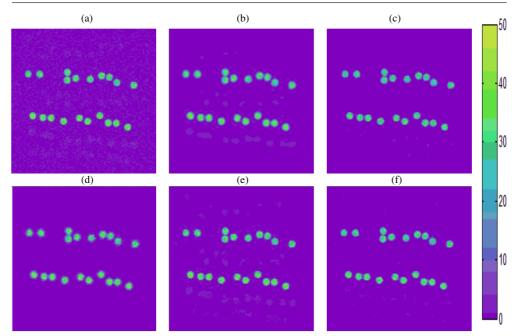
**Figure 9.** The x-ray spectral images at the energy channel of Fe's KL2 line energy (6.39 keV) for (a) original data, (b) BLS-GSM method, (c) ATW-LM method, (d) MPG-ALS method, (e) SURE-LET method and (f) BPR-RR method.
