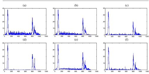
**Figure 8.** Typical single-pixel spectra of the Cu/Zn alloy wire (line c in figure 2(a), the line displayed in figure 7) for (a) original data, (b) BLS-GSM method, (c) ATW-LM method, (d) MPG-ALS method, (e) SURE-LET method and (f) BPR-RR method (vertical axis: photon counts; horizontal axis: eV).
