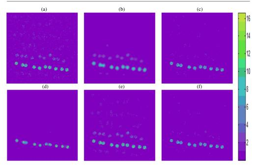
**Figure 3.** The x-ray spectral images at the energy channel of Mn's KL2 line energy (5.89 keV) for (a) original data, (b) BLS-GSM method, (c) ATW-LM method, (d) MPG-ALS method, (e) SURE-LET method and (f) BPR-RR method.
