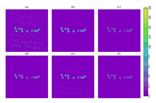
**Figure 7.** The x-ray spectral images at the energy channel of Zn's KL2 line energy (8.62 keV) for (a) original data, (b) BLS-GSM method, (c) ATW-LM method, (d) MPG-ALS method, (e) SURE-LET method and (f) BPR-RR method.
