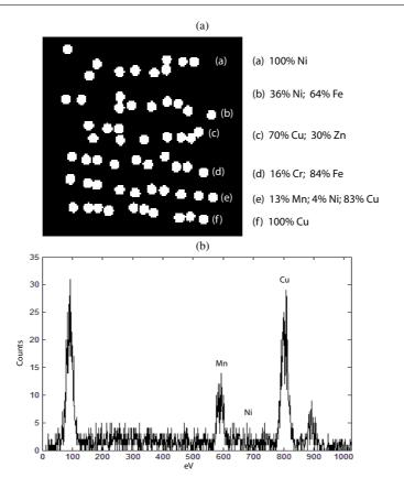
**Figure 2.** (a) The different positions of the wires with the different wire compositions and component concentrations: (a) 100% Ni, (b) 36% Ni, 64% Fe, (c) 70% Cu, 30% Zn, (d) 16% Cr, 84% Fe, (e) 13% Mn, 4% Ni, 83% Cu, (f) 100% Cu ((a)–(f) are referred to the rows of dots in figure 2(a)). (b) A single-pixel spectrum from the Cu/Mn/Ni Wire.
