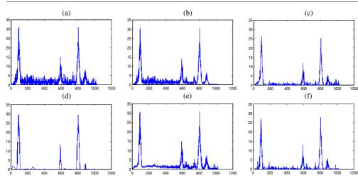
**Figure 4.** Typical single-pixel spectra of Mn/Ni/Cu alloy wire (line e in figure 2(a), the line displayed in figure 3) for (a) original data, (b) BLS-GSM method, (c) ATW-LM method, (d) MPG-ALS method, (e) SURE-LET method and (f) BPR-RR method (vertical axis: photon counts; horizontal axis: eV).
