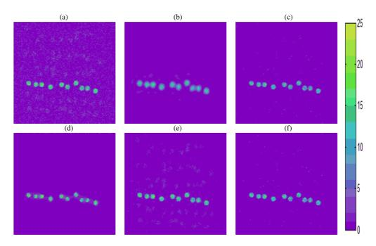
**Figure 5.** The x-ray spectral images at the energy channel of Cr's KL2 line energy (5.41 keV) for (a) original data, (b) BLS-GSM method, (c) ATW-LM method, (d) MPG-ALS method, (e) SURE-LET method and (f) BPR-RR method.
