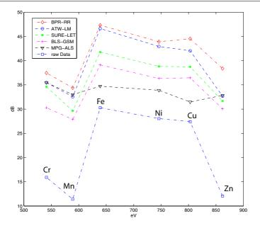
**Figure 10.** The signal-to-noise ratios estimated from the x-ray spectral images of each element's KL2 line energy. The elements from the left to right are Cr (5.41 keV), Mn (5.89 keV), Fe (6.39 keV), Ni (7.46 keV), Cu (8.03 keV) and Zn (8.62 keV).
